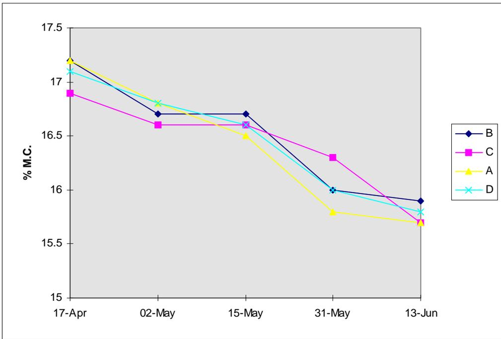
Figure 47 - Moisture contents at the surface of DE treated (A, D) and untreated (B, C) quadrants of a 20 t bin of wheat.
