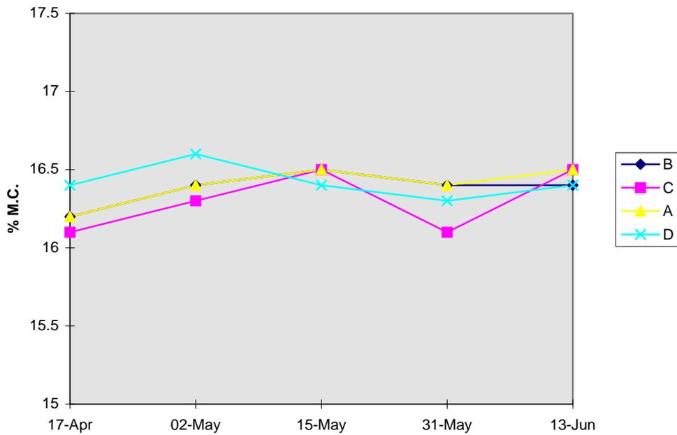
Figure 48.- Moisture contents at a depth of 0.25m in DE treated (A, D) and untreated (B, C) quadrants of a 20 t bin of wheat.
